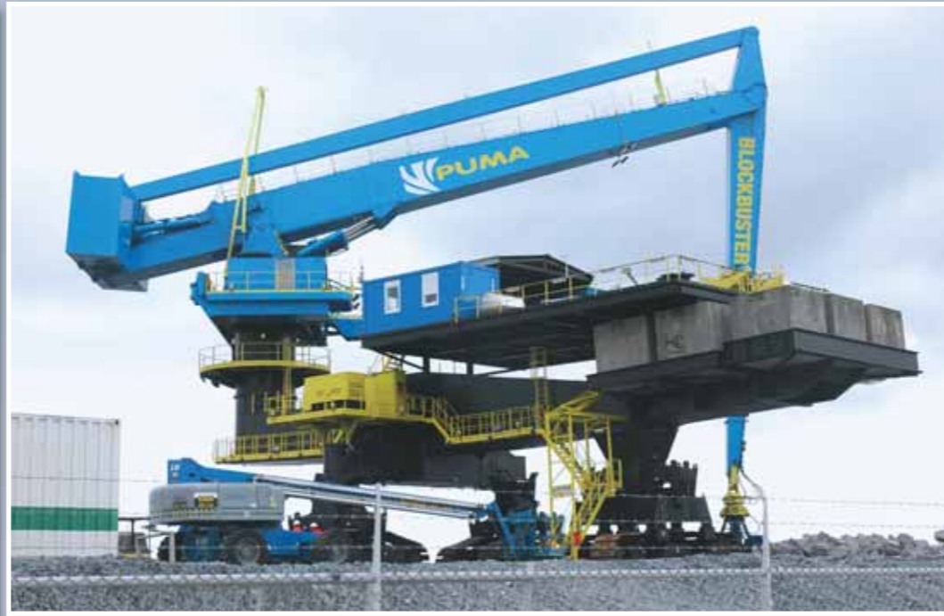
This Picture and Below: Three pairs of track units are needed to support the weight of the 1200-tonne structure, which includes undercarriage ballast weighing around 400 tonnes.
