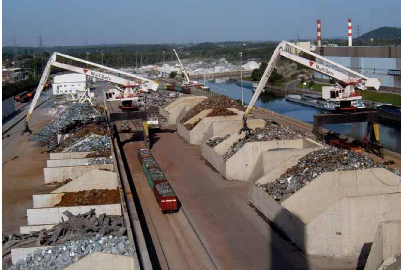
heights of 15m or more. The E-Handler becomes one efficient unit together with, for instance a shredder, and can carry out all tasks involved: unloading trucks, storing material, feeding the shredder as well as loading the processed metals.
