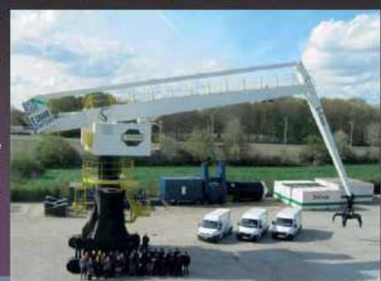
different models with up to 31.7m (104ft) outreach and up to 13.6 metric tonne (15.0 US ton) capacity.
