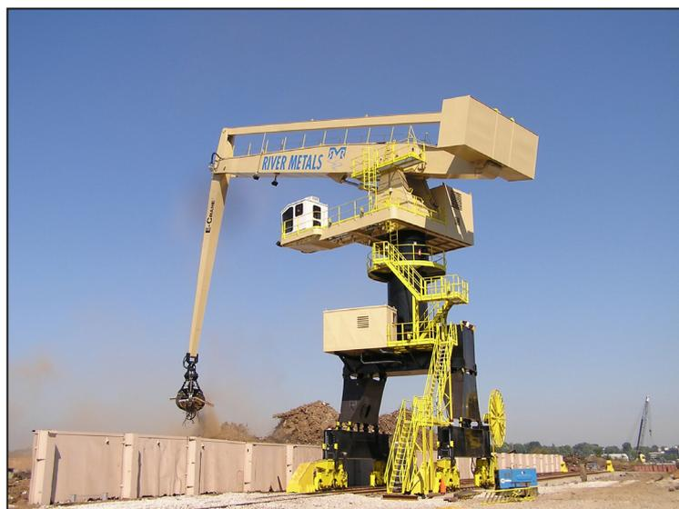
End 2007, River Metals Recycling replaced several conventional material handlers by the 1000 Series E-Crane®, that is now feeding the world's largest shear: the 3000 ton Henschel scrap shear. This brought a lot more flexibility to RMR's operations: in between shear cycles the E-Crane®, unloads trucks, sorts and stockpiles sheared material and in addition to a 4 tine scrap grab, the E-Crane® is also magnet equipped for greater versatility.
