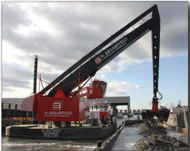
The new E-Dredger® features the renowned E-Crane equilibrium principle for smooth, efficient, energy saving operation in a multitude of dredging and related applications. These include sites where E-Crane customers typically operate, such as piling, ship salvaging, heavy demolition with dynamiting, classic dike works, construction of breakwaters, quay construction, land reclamation, and beach and embankment preservation.
