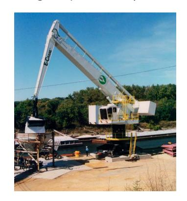
The Cargill Fertilizer facility in Savage Minnesota needed to reduce operating costs and increase the volume produced by their barge offloading operation. A conventional cable crane and rope operated bucket had been the offloading method at "Port Cargill" facility for years but - increasing safety concerns, repair costs and poor reliability made it clear that a change was needed.
